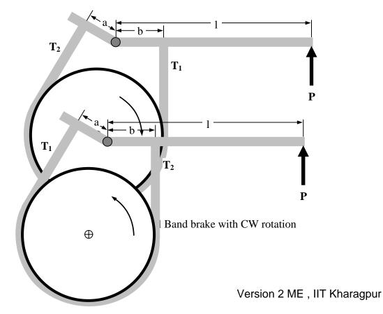
Fig 12.2.2(b): Differential Band brake with CCW rotation
